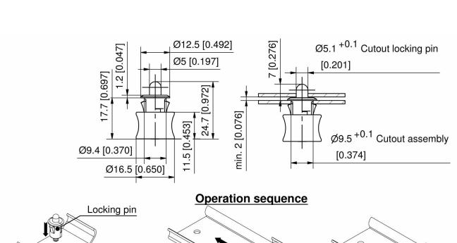
To install, the locking pin is simply pushed into the cutout without the use of tools or hardware. The handle slides over the housing and secures permanently into the groove of the pin.
