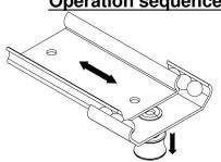
To lock, the spring-loaded handle is released. To loosen, the spring-loaded handle is pulled out.
