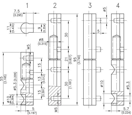
180° Profile-Hinge, Screw-on or Weld-on.
