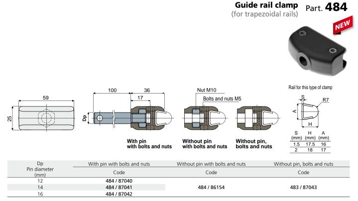
MATERIALS: Clamp made of reinforced polyamide black colour; pin, bolts and nuts made of stainless steel AISI 304.
